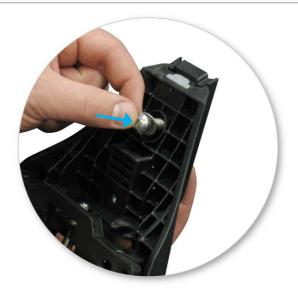
Insert the capscrew and washer together through the back of the leg.
