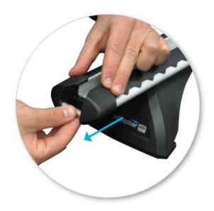
Remove the endcap by pulling on the endcap pin and pushing on the top of the endcap. Use a side to side motion to assist.
