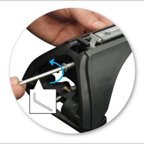
Use the Hex Key to fully undo the adjusting screw.
