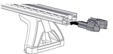
Secure using plastite screw from your TrimHD bar kit. Tighten using a 4 mm hex key.
