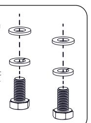
Loosely finger tighten nut plates to legs as shown using the screw assemblies from the previous step.
