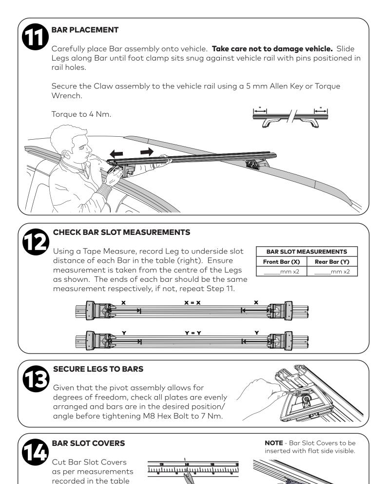
on Step 12 and push into underside channel of front and rear Bar
