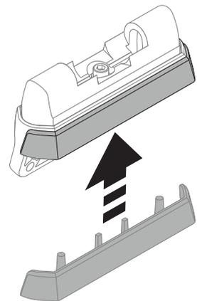
**EN** Install rubber skirt by inserting the four posts into the plastic base just far enough to stay. The spacer height will self adjust in step 3.
