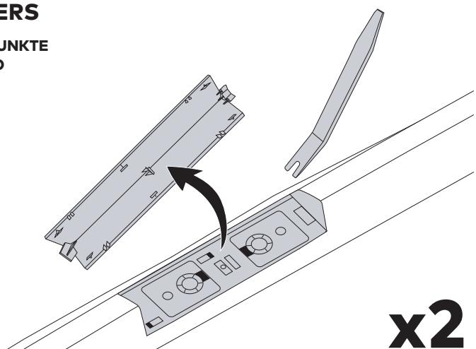
**x2****EN Using a plastic pry tool, carefully pry up and remove each of the 4 covers from the rails on your vehicle.**
