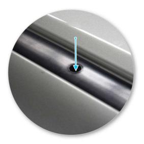
Ensure the hole in rubber ditch mould lines up with mount.
