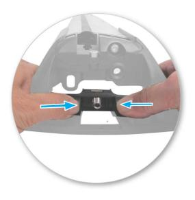
Remove plastic clamp block by gripping bar leg with fingers and push firmly with thumbs until clamp block drops out behind leg.
