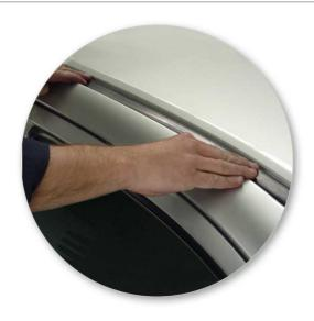
Re-install rubber ditch mould in roof channel.
