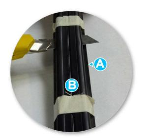
Carefully cut rubber ditch mould between faces along steel strip.
