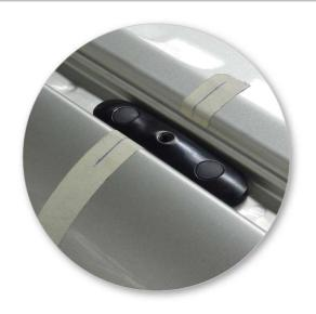
Fit plastic plugs to permanent mount blocks over rivet heads.
