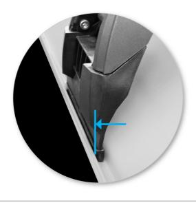
Loosely position crossbar ensuring the guttermount blade is hard against the inside of the vehicle gutter.
