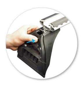
Hold adjusting screw in and slide crossbar in or out as required.
