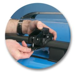
Fit the plastic nut onto the adjustment screw and swing it down under the clamps. Tighten the nut until the clamp just touches the underside of the siderail.
