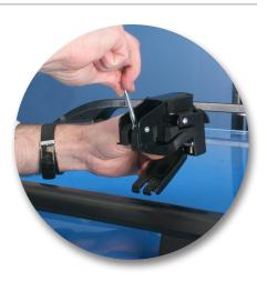
Fit the leg and clamp assembly to the vehicle side-rail taking care to hold the adjustment screw clear of the rail.
