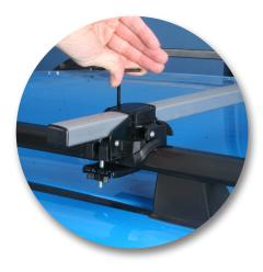
Using the hex key, tighten up the 2 screws in each leg at the rear, taking care to tighten both sides evenly.
