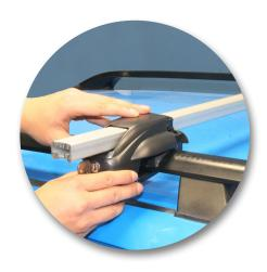
Slide the covers onto the legs. Lock, using the key.
