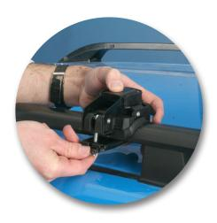
Fit the plastic nut onto the adjustment screw and swing it down under the clamps. Tighten the nut until the clamp just touches the underside of the siderail.
