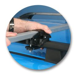
Slide the crossbars through the legs and even up the amount of crossbar that protrudes through the legs on both sides of the vehicle.
