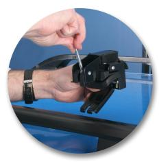
Fit the leg and clamp assembly to the vehicle side-rail taking care to hold the adjustment screw clear of the rail.
